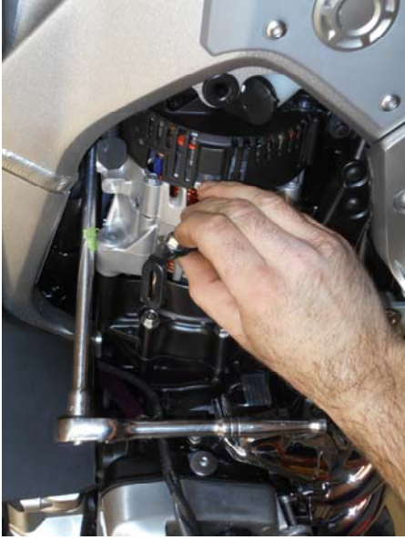
38 upper shock clevis bolt
